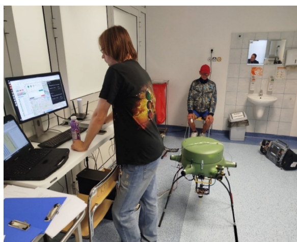
Fig. 3. Performing non-contact vital signs measurement using noise radar
